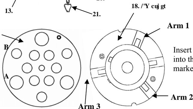
Insert the wires of lamp socket into the appropriate male plugs marked with labels (L) and (N)
